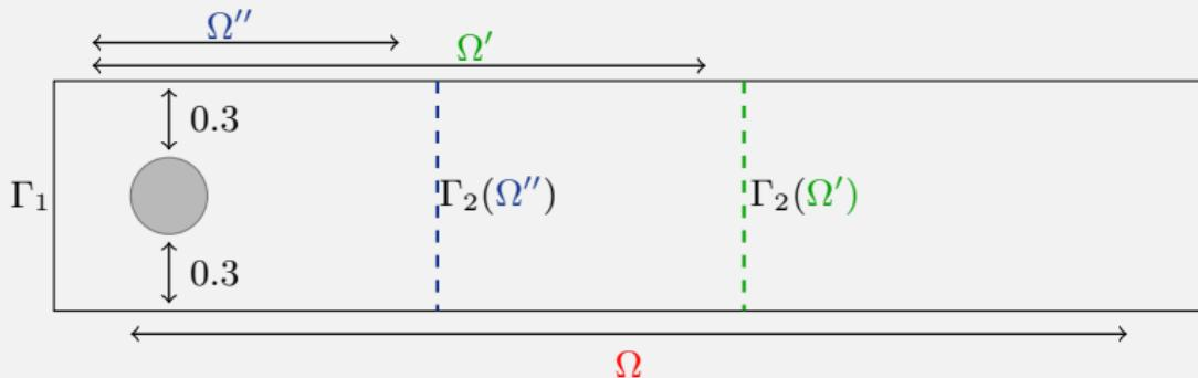
$$\Omega = [0, 5] \times [0, 1] \rightarrow 12118 \text{ cells}, \quad \Omega' = [0, 3] \times [0, 1] \rightarrow 8636 \text{ cells}$$
