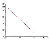
$\Rightarrow$  Second-order accuracy in the  $L^2$ -norm w.r.t. the mean distance between two connected interface-markers
