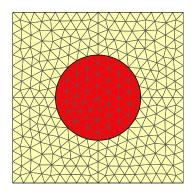
Laplace uniform capillary pressure  $p_c = \sigma \kappa = \sigma/R = 400 \, Pa$  (whatever density) in a disk droplet of radius  $R = 2.5 \, 10^{-3} \, m$  for a constant surface tension  $\sigma = 1 \, N/m$  (no gravity force, only the capillary force  $f_c := \sigma \, \kappa \, \nabla \xi$  on  $\Sigma$ )
