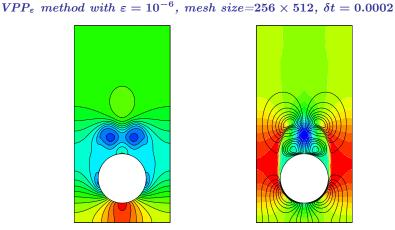
Cylinder diameter d = 0.05,  $\rho_s = 10^6$ ,  $\rho_f = 1$ ,  $\mu_s = 10^{12}$ ,  $\mu_f = 10^{-5}$ , domain  $0.1 \times 0.2$ , cylinder initially with no motion at height y = 0.15.
