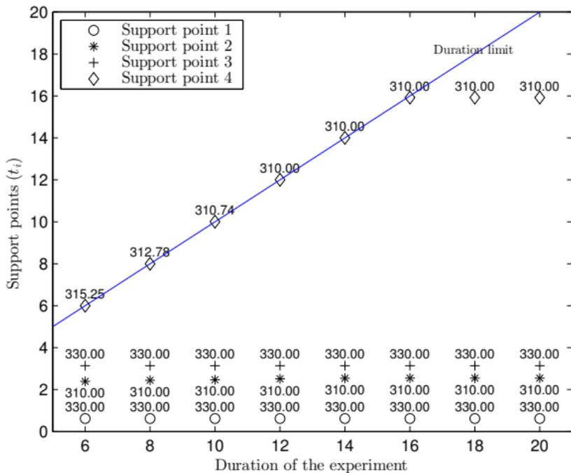
Support points of designs with four batches as  $t^{\text{UP}}$  increases. The values close to the support points are the respective temperatures
