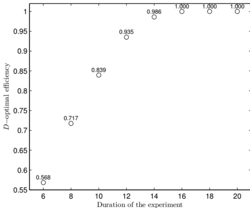
D-efficiency of designs for four batches for different interval durations
