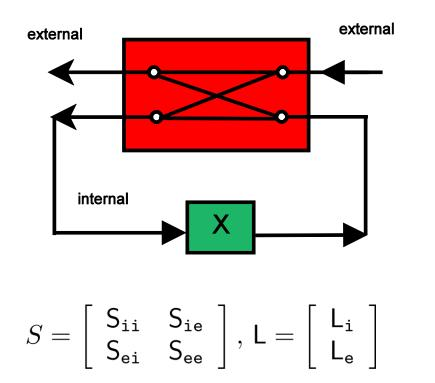
The reduced model obtained by eliminating all the internal channels (instantaneous feedback) is determined by the operators  $(S^{fb}, L^{fb}, H^{fb})$  given by
