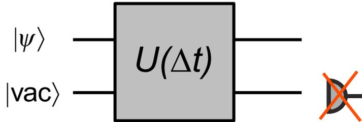
$$\frac{d}{dt} \rho(t) = -i[H_{\text{sys}}, \rho(t)] + \frac{1}{2} \gamma (2c\rho(t)c^\dagger - c^\dagger c\rho(t) - \rho(t)c^\dagger c)$$
