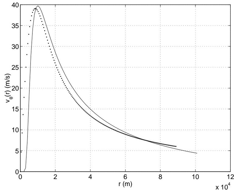
Comparison between the Holland's empirical model for  $v_\theta$  (continuous line) and our result (dotted line).
