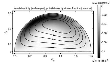
Figure 5. Surface plot of the (dimensional) toroidal vorticity  $\omega_\theta$  combined with contours of the poloidal velocity stream function  $\psi$  with  $M = 8.64 \times 10^{-3}$ . The grey-scale bar indicates the dimensional value of the toroidal vorticity in  $\text{s}^{-1}$ . Stress-free boundary conditions are assumed.
