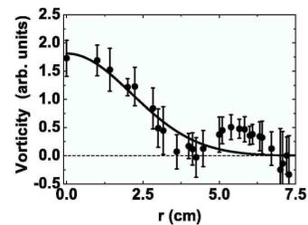
FIG. 3. Vorticity as a function of radius. The solid curve indicates the vorticity distribution given by Eq. (1), where  $\Gamma = 7.7 \times 10^7 \text{ cm}^2/\text{s}$  and  $l = 3.0 \text{ cm}$ .
