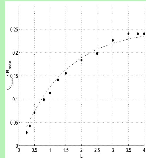
$$\frac{r_{v_{\theta}^{\max}}}{R_{\max}} = \frac{1}{4} \left[ 1 - \exp\left(-\frac{R_{\max}}{2}\right) \right]$$
