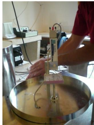
Sparse measures of magnetic field  $\mathbf{B}[\mathbf{m}]$  (magnetometer)
