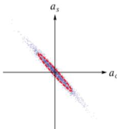
b) amplitude squeezing (10 dB,  $\phi = \frac{\pi}{2}$ ,  $A_c = 5$ )
