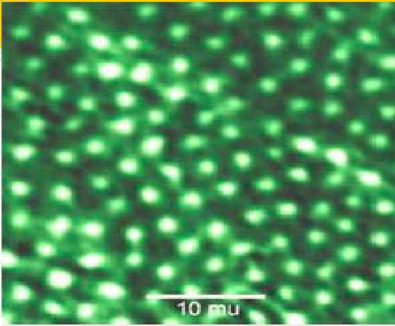
**Quantized Vortex** in a type-II superconductor
