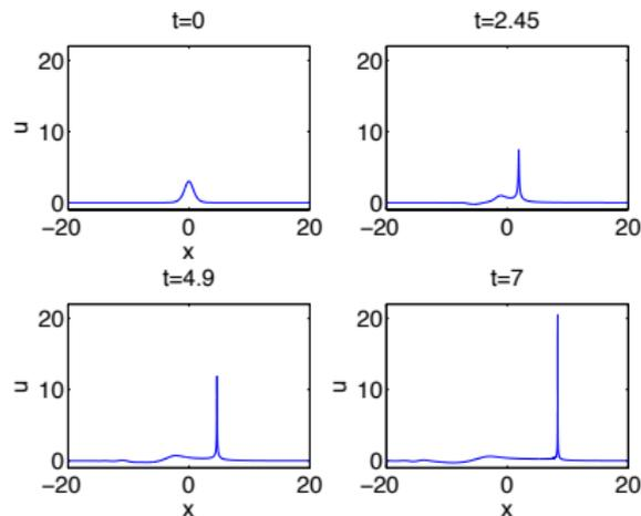
FIGURE 4. Solution to the fKdV equation <sup>(Cauchy)</sup> (17) for  $\alpha = 0.5$  and the initial data  $u_0 = 3\operatorname{sech}^2 x$  for several values of  $t$ .
