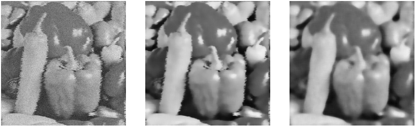
Figure: Dejittering: the results of algorithms from damped second order TVF (middle) and damped second order level sets MCF (right).
