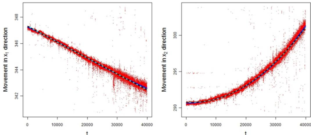
Under the hypothesis of a (low order) polynomial drift, very narrow simultaneous confidence intervals (due to a much larger number of pixel data than of bead data).
