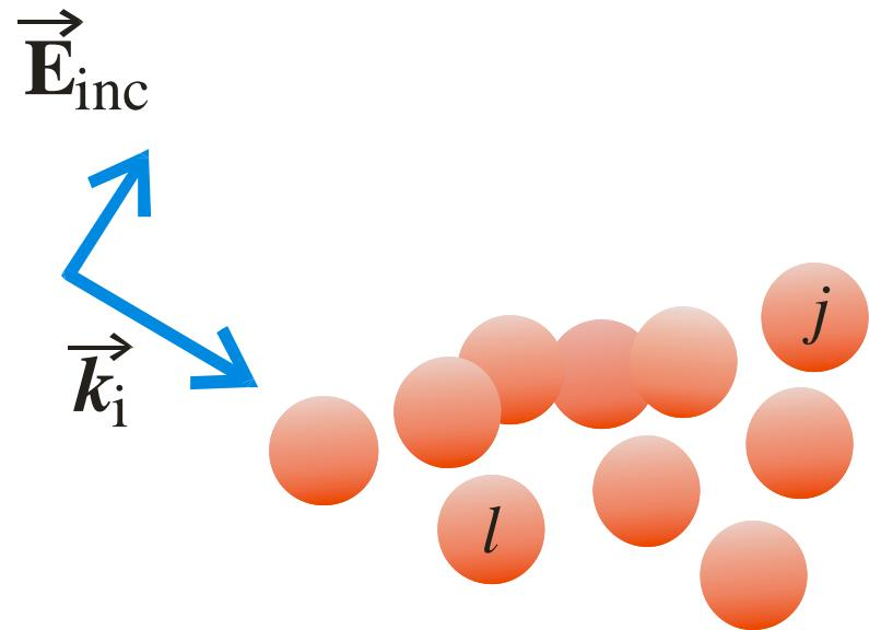
$$\begin{bmatrix} [T^{(1)}]^{-1} & -H^{(1,2)} & \dots & -H^{(1,N)} \\ -H^{(2,1)} & [T^{(2)}]^{-1} & \dots & -H^{(2,N)} \\ \vdots & \ddots & \ddots & \vdots \\ -H^{(N,1)} & -H^{(N,2)} & \dots & [T^{(N)}]^{-1} \end{bmatrix} \begin{bmatrix} f^{(1)} \\ f^{(2)} \\ \vdots \\ f^{(N)} \end{bmatrix} = \begin{bmatrix} a^{(1)} \\ a^{(2)} \\ \vdots \\ a^{(N)} \end{bmatrix}$$
