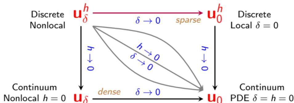
AC scheme: monolithic discretization of heterogeneous (local/nonlocal) models
